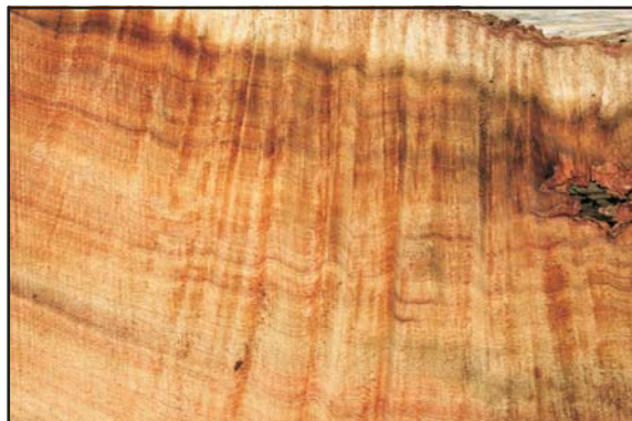
Older koa wood commonly shows curl, particularly near branch unions. With heavy curl, koa wood can be valued at up to $100 per board foot.
